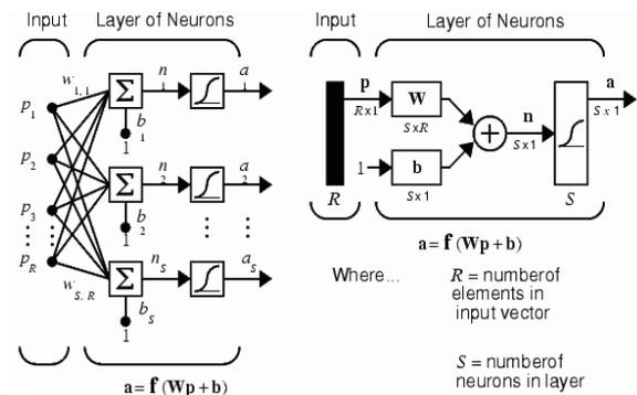
Fig. 2. Feed forward Network
