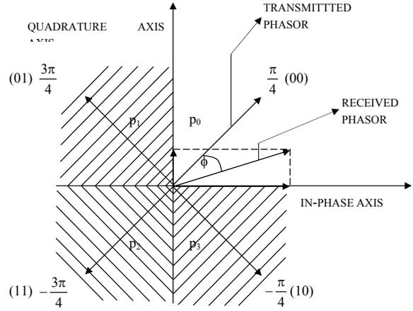
Fig. 4. Detection of a quaternary PSK signal when the transmitted bit pair is 00
