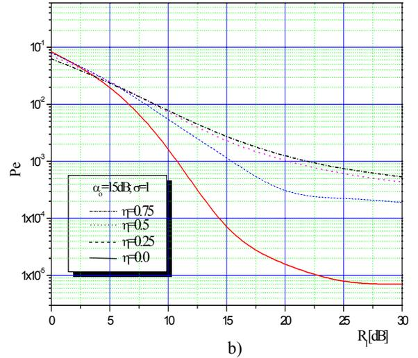
**Fig. 3.** Average error probability performance of a QPSK coherent detector with a noisy carrier synchronization reference signal: a) when  $\alpha_0$  is a parameter, while  $\eta$  and  $\sigma$  are constants; b) when  $\eta$  is a parameter, while  $\alpha_0$  and  $\sigma$  are constants
