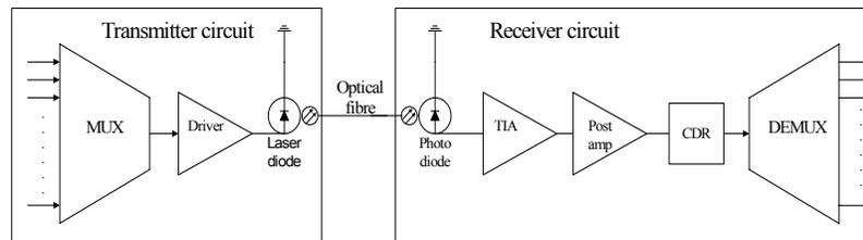
Fig. 1. Building blocks of optical communication system
