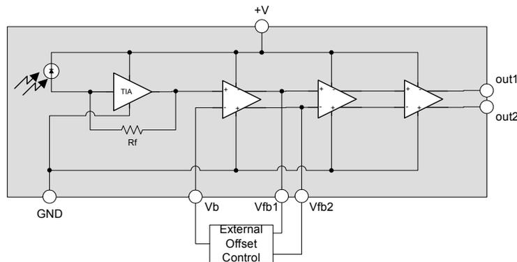
Fig. 2. Block diagram of TIA
