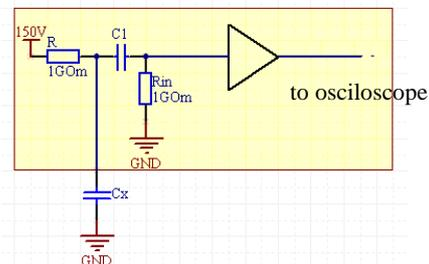
**Fig. 16.** Scheme of capacitance transformation into voltage.  $C_x$  – transducer capacitance
