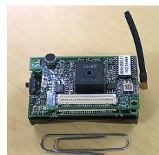
Fig. 1. Smart dust mote MicaZ from Crossbow Technology
