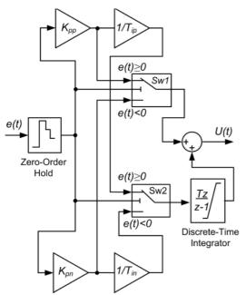
Fig. 1. The block diagram of digital aPI controller
