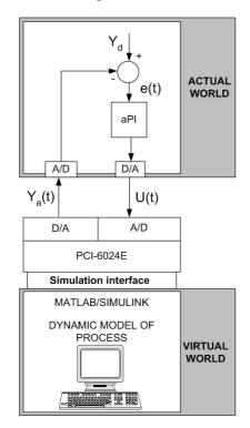
**Fig. 2.** The block diagram of the HIL simulation system for the investigation of aPI controller
