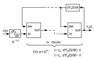
Fig. 4. The model of the *m*-order process with the asymmetric dynamics and response delay for the software Simulink
