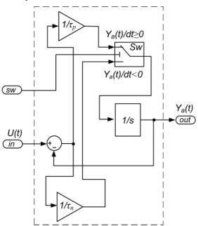
Fig. 3. The model of 1-st orders process with the asymmetric dynamics for the software Simulink
