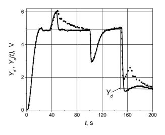
**Fig. 6.** Set point pulse and load disturbance response of the control system based on the aPI (solid line) and PI (doted line) controllers. The PI controller parameters ( $K_p$ =0.8,  $T_i$ =10s) are adjusted to dynamics of the process, which corresponds to the rise of controlled parameter. Parameters of aPI controller:  $K_{pp}$ =0.8,  $K_{pn}$ =0.5,  $T_{ip}$ =10s,  $T_{in}$ =2s
