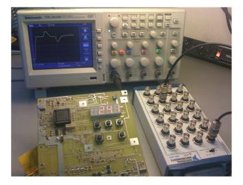
**Fig. 5.** The HIL simulation system for the investigation of aPI controller (the aPI controller is on the left, the connector block of multifunctional PC board PCI-6024E, which is connected to the PC with the installed Simulink software– on the right)
