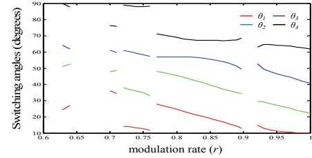
**Fig. 6.** Switching angles versus  $r$  leading to the lowest THD
