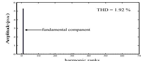
**Fig. 14.** Frequency content of the stator current of the asynchronous machine fed by a 9-level USAMI controlled by the proposed neural HES
