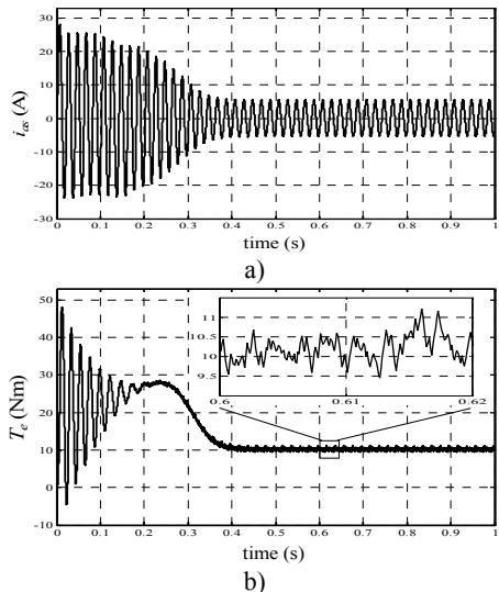
**Fig. 11.** Stator current (top) and electromagnetic torque (bottom) of the asynchronous machine fed by a 9-level USAMI controlled by the MCPWM
