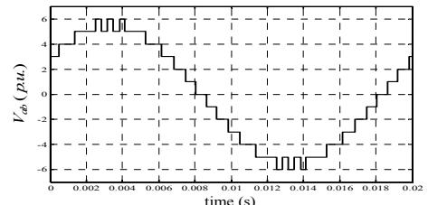
**Fig. 9.** Output voltage  $V_{ab}$  of the 9-level USAMI controlled by the proposed neural HES (with  $r(l) = 0.8$  and  $p = 4$ )
