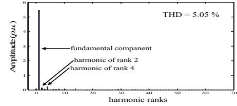
**Fig. 12.** Frequency content of the stator current of the asynchronous machine fed by a 9-level USAMI controlled by the MCPWM
