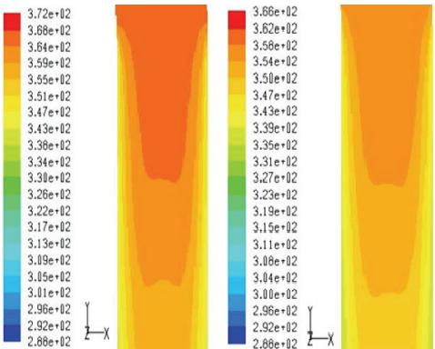
**Fig. 9.** Temperature contours at the entrance of the cooling region
