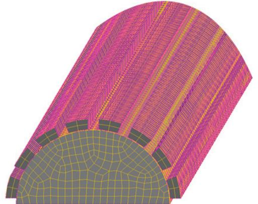
**Fig. 4.** Computational mesh for the water domain
