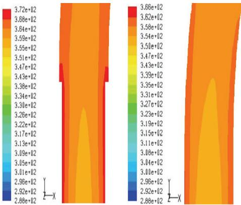
**Fig. 8.** Temperature contours at exit of the hot region
