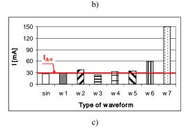
**Fig. 3.** Tripping current of the RCD6:  $I_{\Delta n} = 30$  mA, type AC; residual current comprises: a)  $1^{st}$  and  $3^{rd}$  harmonics, b)  $1^{st}$  and  $49^{th}$  harmonics, c) several harmonics
