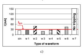
**Fig. 4.** Tripping current of the RCD15:  $I_{\Delta n} = 30$  mA, type A; residual current comprises a)  $1^{st}$  and  $3^{rd}$  harmonics, b)  $1^{st}$  and  $49^{th}$  harmonics, c) several harmonics
