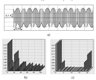
**Fig. 2.** Earth fault current (a) in case of fault in the output terminals of the frequency converter (TCad simulation) and its spectrum of harmonics (b, c). Motor frequency 50 Hz, PWM frequency 1 kHz
