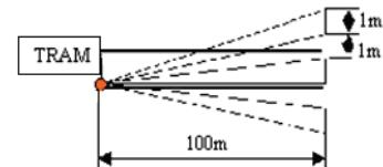
**Fig. 3.** LIDARs beam geometry
