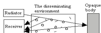
Fig. 1. LIDARs working principle
