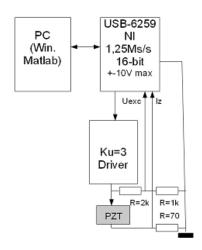
Fig. 1. Measurement setup (block diagram)
