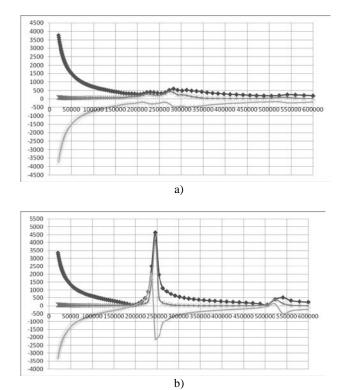
Fig. 3. Bonded (S3): a – vs. free(Sx); b – PZT impedance
