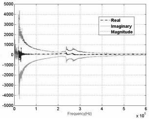
**Fig. 7.** PZT (S3) impedance obtained by the aid of a chirp (80ms) signal
