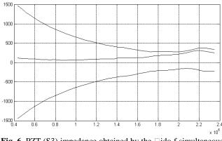
**Fig. 6.** PZT (S3) impedance obtained by the  $\Box$  ido f simultaneous multi-frequency method, by using 4x FFT and <sup>1</sup>/<sub>4</sub> shift of frequency values
