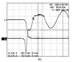
**Fig. 3.** The waveforms of the voltage arc and current arc in the case of quartz sand (a) and silicon carbide (b)
