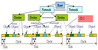
**Fig. 3.** The structure of the acquisition cycle, executed by the communication tasks, excepting CANOpen
