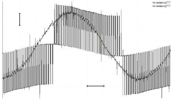
**Fig. 3.** Phase current and voltage diagrams of the loaded standard 0,75 kW motor with copper rotor winding supplied from Altivar 16: horizontal segment corresponds to 2,5 ms, vertical – to voltage of 100 V and current of 6 A; zeroes of voltage and current diagrams are not matched
