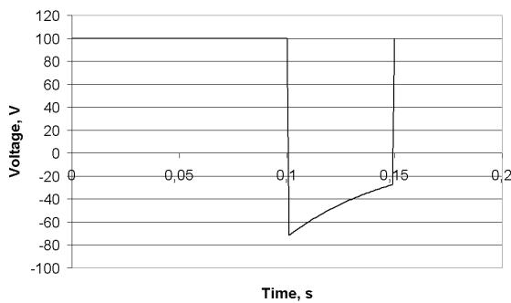
**Fig. 6.** Variation of the voltage drop over resistor  $R_2$  during the commutation period
