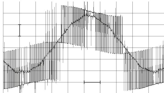
**Fig. 2.** Phase current and voltage diagrams of the loaded standard 0.75 kW motor supplied from Altivar 16: horizontal segment corresponds to 2,5 ms, vertical – to voltage of 100 V and current of 6 A; zeroes of voltage and current diagrams are not matched
