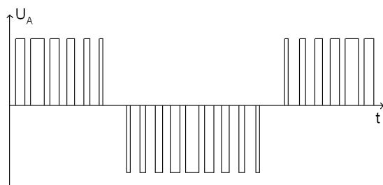
**Fig. 1.** Phase voltage at the output of the inverter under active load
