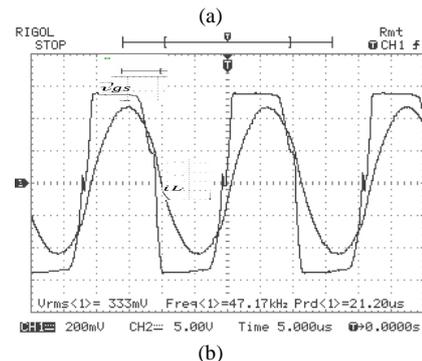
Fig. 6. Load current and driving voltage results: (a) simulation; (b) experiment (CH1:  $i_L$  (100mV  $\equiv$  1A), CH2:  $V_{gs}$ ).
