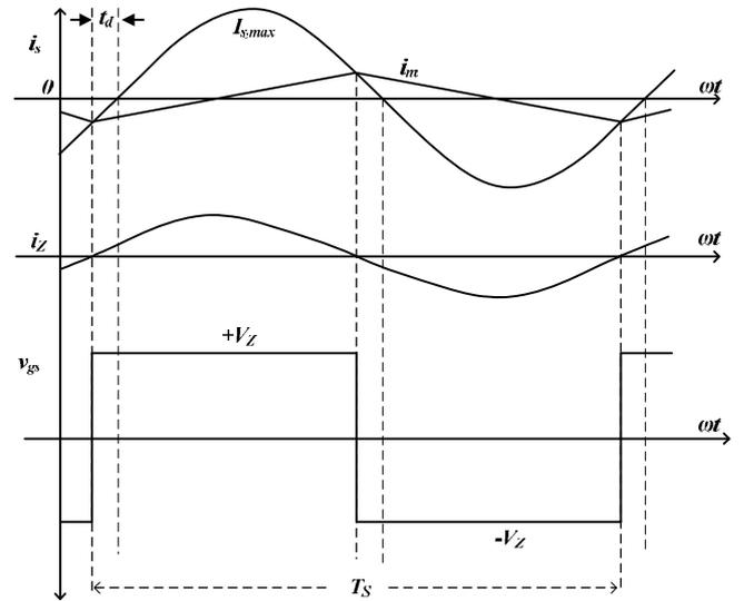
Fig. 3. Theoretical waveforms of the driver circuit.
