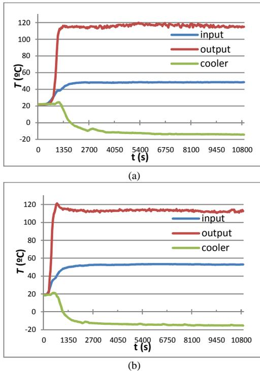
Fig. 7. Temperature curves of absorption cooler: (a) the resistance heated absorption cooler; (b) the induction heated absorption cooler.
