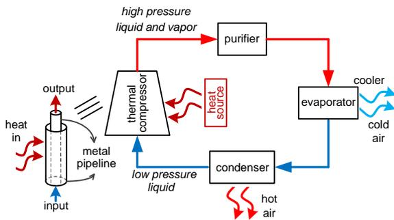
Fig. 4. Simplified cooling cycle of the absorption cooler.
