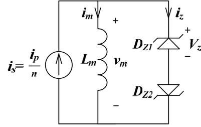
Fig. 2. Linear model of the current transformer.
