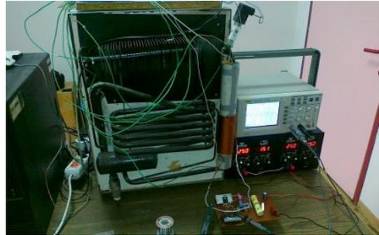
Fig. 5. Self oscillated induction heater and absorption cooler.
