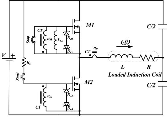
Fig. 1. Self oscillating half bridge resonant inverter.
