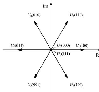
Fig. 2. Voltage space vectors generated by three-phase inverter.
