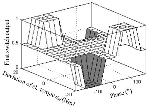
Fig. 7. First switch output dependence from deviation of electromagnetic torque and phase.
