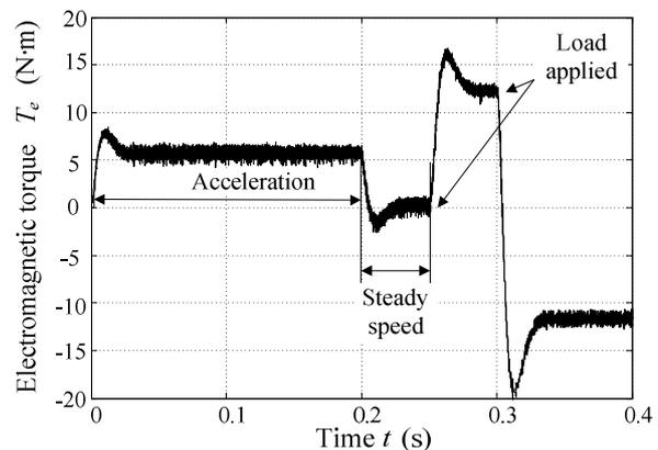
Fig. 10. Electromagnetic torque of DTFC induction drive.
