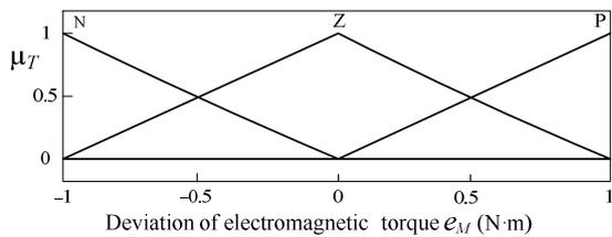
Fig. 5. Membership functions of torque deviation fuzzification block.
