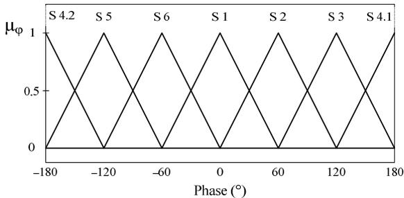
Fig. 6. Membership functions of phase fuzzification block.
