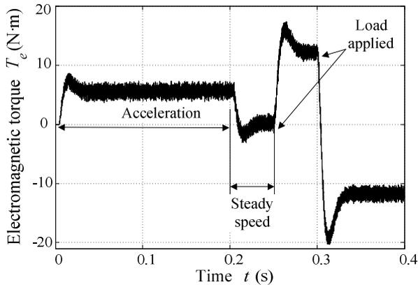
Fig. 11. Electromagnetic torque of traditional DTC induction drive.
