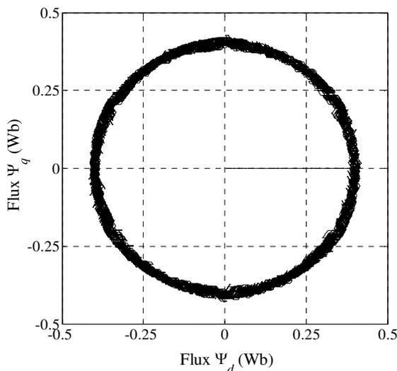
Fig. 12. Stator flux trajectory of traditional DTC.
