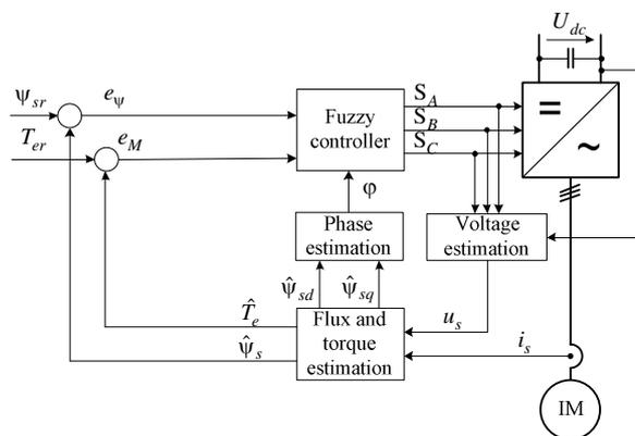
Fig. 1. DTFC scheme for induction motor drives.
