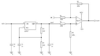
Fig. 3. Block scheme of circuit for voltage adjustment.
