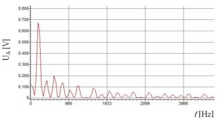
Fig. 13. Amplitude spectrum of square waveform.
