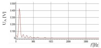
Fig. 11. Amplitude spectrum of triangual waveform.
