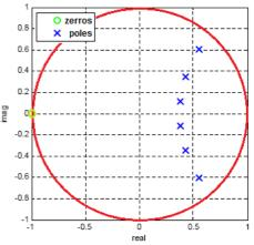
Fig. 5. Distribution of poles and zerros of proposed filter.
