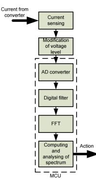
Fig. 1. Block scheme of system for analysis of recuperative currents.
