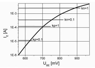
Fig. 2. Experimental voltage-current characteristic of the base-emitter junction of the p-n-p integral lateral transistor with junction area  $1.3 \times 10^{-4}$  mm<sup>2</sup>.
