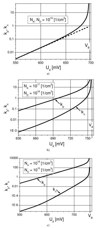
Fig. 1. Dependences of minority carrier hole and electron injection levels on voltage drop across the depletion region for silicon junctions No1–No.3 calculated using equations (9) and (10) (solid lines). The dependence for junction No1 presented by the dashed line has been calculated using equations (5) and (6).
