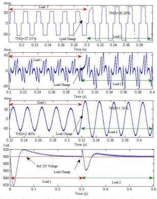
Fig. 4. Performance of the APF under ideal grid voltage and step-up load change. Top waveform: Load current of phase a. Compensating current of phase a. Grid current of phase a. Bottom waveform: DC link capacitor voltage.
