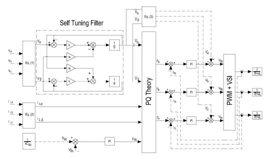
Fig. 2. The block scheme of the proposed control system.
