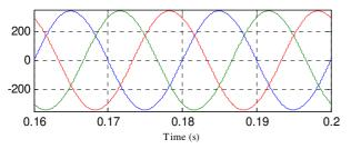
Fig. 3. Three phase balanced and undistorted (ideal) grid voltages.
