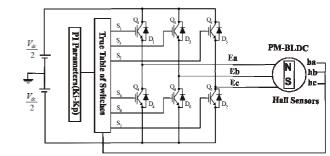
Fig. 1. Block diagram of PM-BLDC with IGBT based inverter.
