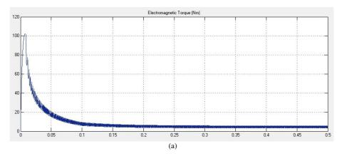
The moment of inertia value taken for this case is 0.0089 kg/m<sup>2</sup> and it reaches steady state speed at time 0.25 seconds
