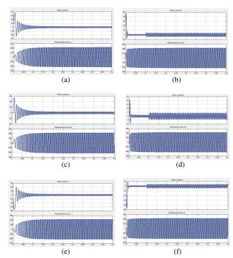
Fig. 3. Currents and Back-EMF changes with inertia of moment (a)  $i_a$  current with  $emf_a$  at 0.0089 kg/m<sup>2</sup> inertia (b)  $i_a$  current with  $emf_a$  at 0.00091 kg/m<sup>2</sup> inertia (c)  $i_b$  current with  $emf_b$  at 0.0089 kg/m<sup>2</sup> inertia (d)  $i_b$  current with  $emf_b$  at 0.00091 kg/m<sup>2</sup> inertia (e)  $i_c$  current with  $emf_c$  at 0.0089 kg/m<sup>2</sup> inertia (f)  $i_c$  current with  $emf_c$  at 0.00091 kg/m<sup>2</sup> inertia.
