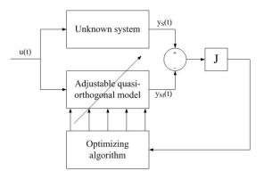
Fig. 2. .Block diagram of the modelling process.
