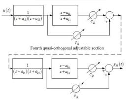
Fig. 9. Quasi-orthogonal model of the laboratory cascade-connected system.
