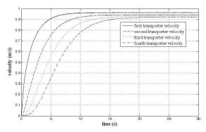
Fig. 8. Step response of laboratory cascade-connected system.
