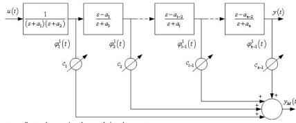
Fig. 1. Adjustable, Legendre type, first order quasi-orthogonal signal generator.
