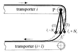
Fig. 5. Rubber transition between transporters.
