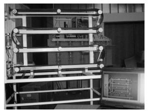
Fig. 7. Laboratory setup - cascade-connected system with four transporters.
