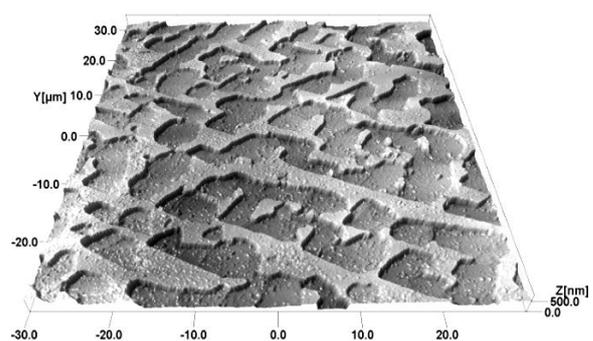
Fig. 1. AFM picture of silicon surface after elimination of Al DW contact.
