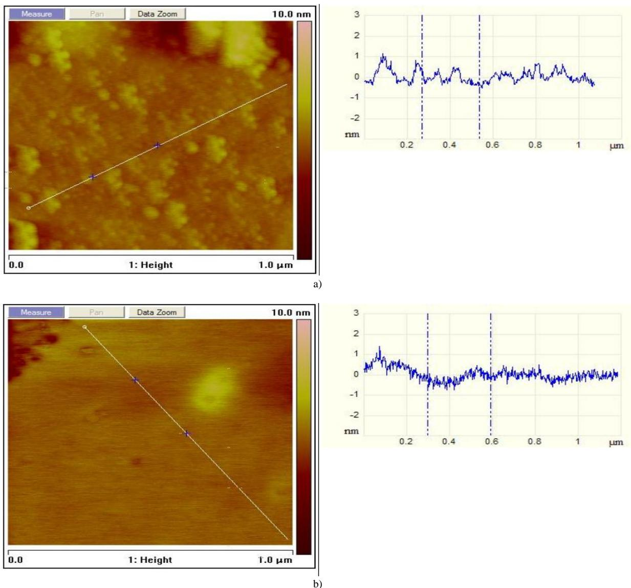
Fig. 2. AFM images and cross-sectional profiles before (a) and after diffusion welding (b).
