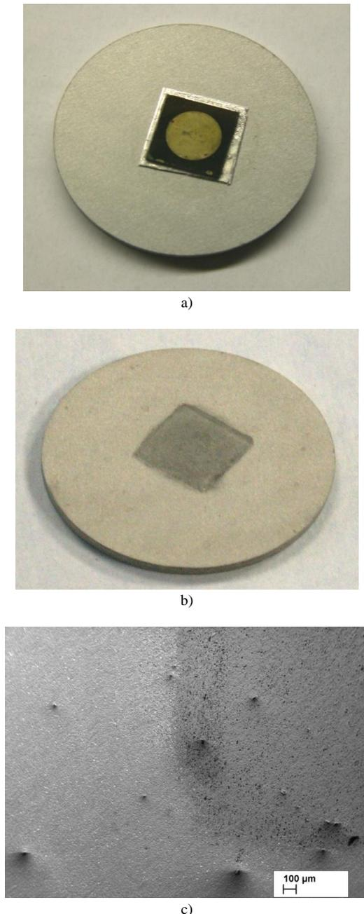
Fig. 3. The view of the welded chip (a), tungsten electrode after etching (b) and tungsten electrode surface under the great magnification (c) (secondary electron image).
