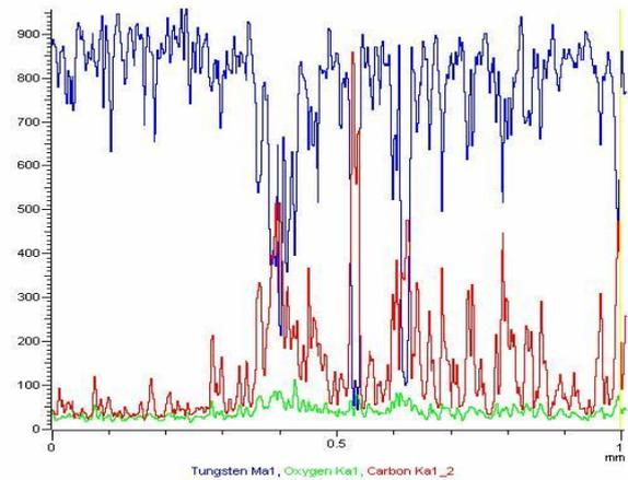
Fig. 4. The spectral distribution of elements on the surface of tungsten in welding area.
