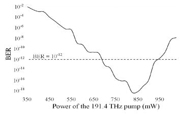
Fig. 4. Dependence of system maximal BER values on the power of the 191.4 THz pump at constant total pump power of 1350 mW.
