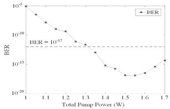
Fig. 3. Dependence of system maximal BER values on the total pump power for 191.4 THz and 194.6 THz pumps frequencies.
