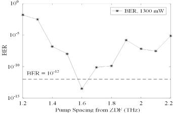
Fig. 2. Dependence of system maximal BER values on the spacing between the pumps and the zero dispersion frequency at equal pump powers and 1.3 W total pump power.
