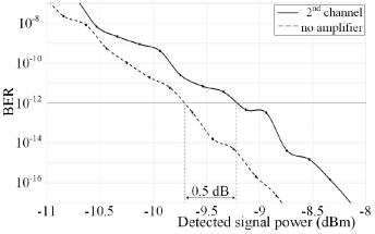
Fig. 6. Dependence BER values on the power of the received signal in the  $2^{nd}$  channel of the system with the dual-pump FOPA (solid line) and in the system without amplification (dashed line).
