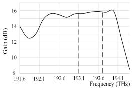
Fig. 5. Gain spectrum ensured by the dual-pump FOPA with the chosen configuration (191.4 THz 675 mW and 194.6 THz 675 mW pumps).
