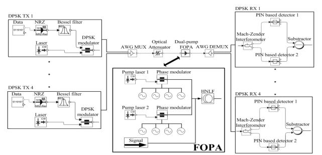
Fig. 1. Simulation model of 4-channel 40 Gbps WDM transmission system with BDPSK modulation format and dual-pump FOPA for loss compensation.
