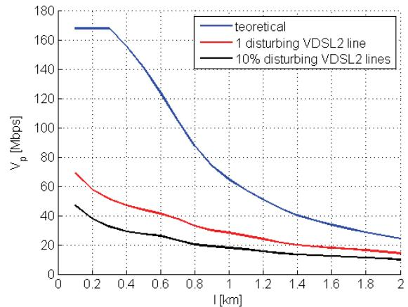
**Fig. 9.** Transmission rate VDSL2 line, frequency band plan B8-12 for downstream direction
