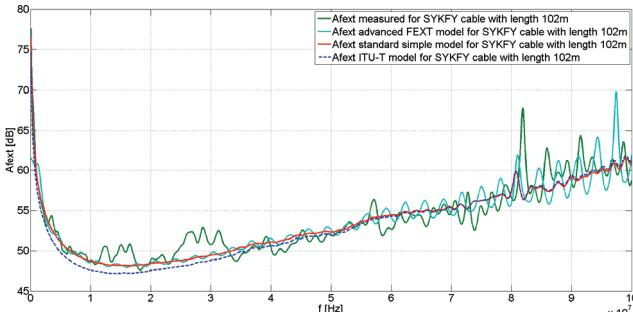
**Fig. 7.** The advanced FEXT model, both standard models and measured characteristic for SYKFY cable
