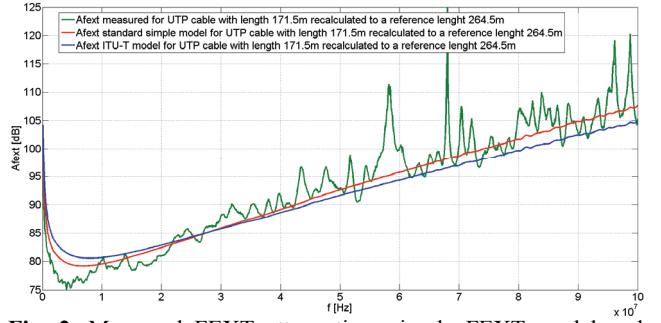
Fig. 2. Measured FEXT attenuation, simple FEXT model and ITU-T model for a UTP cable with length 171.5 m recalculated to a ref. length 264.5 m
