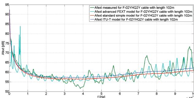
**Fig. 8.** The advanced FEXT model, both standard models and measured characteristic for F-02YHQ2Y cable
