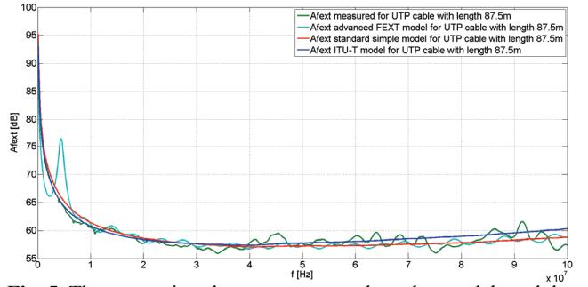
Fig. 5. The comparison between measured results, models and the advanced FEXT model for the length of a cable 87.5 m
