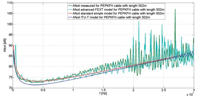
Fig. 6. The advanced FEXT model, both standard models and measured characteristic for PEPKFH cable
