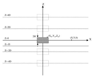
**Fig. 2.** Arrangement of cylinder-shaped current electrodes in the model of three-dimensional resistive medium of finite thickness, restricted by parallel planes Z=0 and Z=-D. *Y*-axis is perpendicular to plane *XZ*
