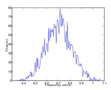
Fig. 5. Distribution of milk conductivity measurement results
