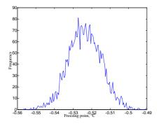
Fig. 6. Distribution of milk freezing point measurement results
