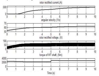
Fig. 6. Curves of the converter's parameters at the jump of wind velocity  $v_w$  ( $U_{vw}$ =0,5 V,  $v_w$ =10÷14 m/s, o t=5 s)
