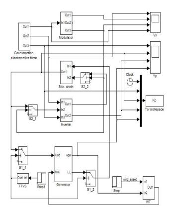
Fig. 3. Mathematical model for the WT's power conversion
