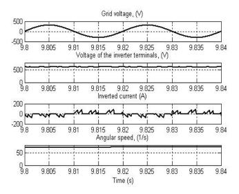
Fig. 5. Curves of the converter's parameters when control voltage of the short-circuiting unit  $U_{vt}=3$  V
