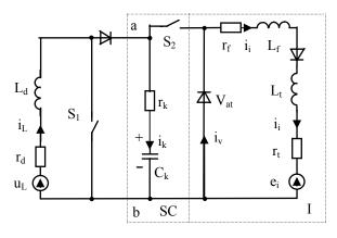
Fig. 2. Equivalent scheme of the power converter
