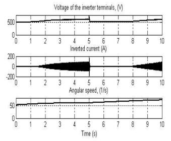
**Fig. 4**. Curves of the converter's parameters at jump of the control voltage  $U_{vtt}$  ( $U_{vtt}$ =0,5÷3 V, o *t*=5 s)
