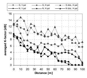
**Fig. 6.** Average Ricean K-factor vs. distance and polarisation for 802.11g and 802.11n devices in long corridor
