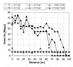
Fig. 5. Client receiving distance and bandwidh estimation to AP
