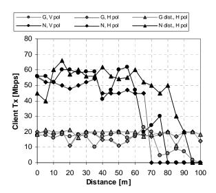
Fig. 4. Client transmiting distance and bandwidth estimation to  $\ensuremath{\mathsf{AP}}$
