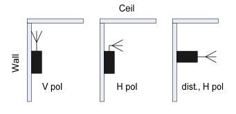
Fig. 2. AP setup for corridor measurements
