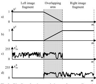
Fig. 9. Blending functions and image fragment line pixel intensities
