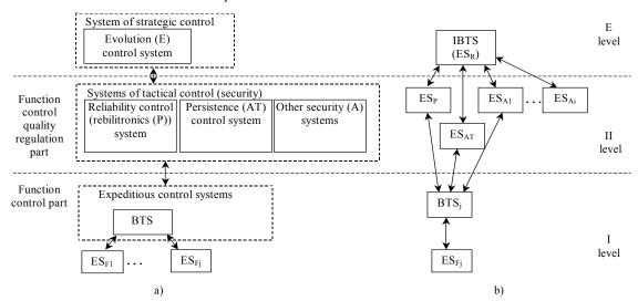
Fig. 5. IBTS control levels (F<sub>i</sub> – j-th purpose function) (a – two-part IBTS; b – symbolic levels of IBTS)
