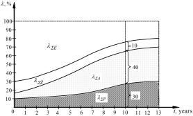
**Fig. 1.** The dynamics of failure intensity due to different factors;  $\lambda_{\Sigma E}$ ,  $\lambda_{\Sigma Z}$ ,  $\lambda_{\Sigma A}$ ,  $\lambda_{\Sigma P}$  – the ES failure intensities conditioned by electronic devices, human-operator, operation algorithms and software
