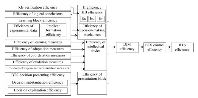
Fig. 7. Integration scheme of efficiency features ( $E_D$ ,  $E_M$ ,  $E_T$  – efficiencies of data, metaknowledge and rules)
