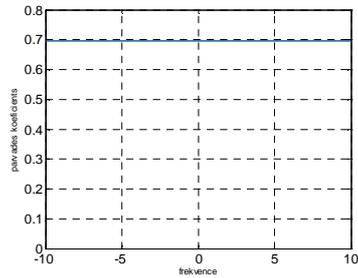
Fig. 11. Transmission coefficients for shielded device
