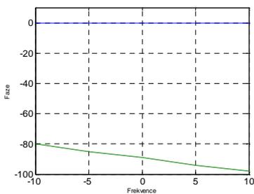
Fig. 12. Transmission coefficients for shielded device phase
