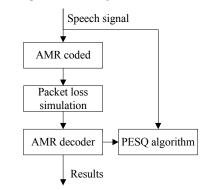
Fig. 3. Simulation scheme
