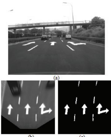
**Fig. 2.** a – Image obtained from the camera perspective; b – image after inverse perspective transformation; c – logic transformed image equivalent [16]
