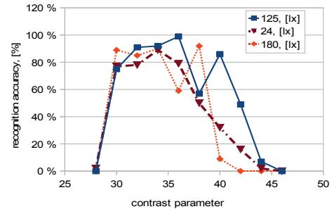
Fig. 6. The functional relationship between contras value, lightening conditions and recognition accuracy
