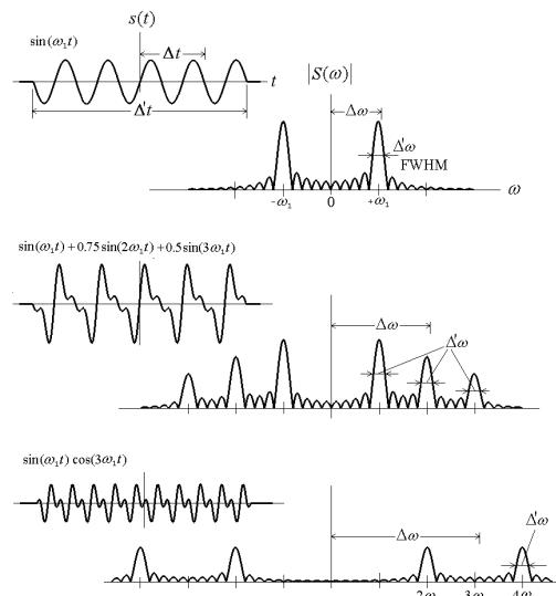
**Fig. 1.** The problematic tasks of pulse train signal (left) to Fourier spectrum (right) transforms for what the conventional methodology yields artificially increased uncertainty product values. The standard deviations  $\Delta t, \Delta \omega$  are shown in comparison with one possible alternative definition: full pulse train duration in time domain  $\Delta' t$  and the full width at half maximum (FWHM) of main spectral peaks  $\Delta' \omega$ .
