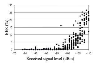
Fig. 3. BER as a function of received signal level
