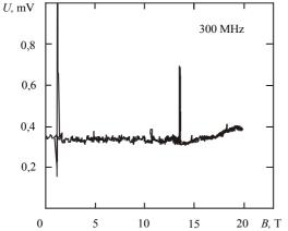
**Fig. 2.** The pick-up signal in milivolts versus constant magnetic field induction *B* in Tesla (pumping 300 MHz)
