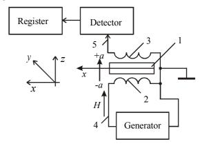
Fig. 1. The experimental device of Helicon Maser
