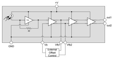
Fig. 2. Block diagram of TIA
