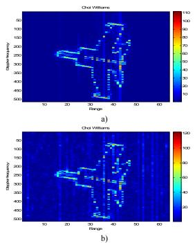
**Fig. 7.** Choi Williams (CW) distribution based ISAR image formation for (a) SNR=10 dB and (b) SNR=0 dB
