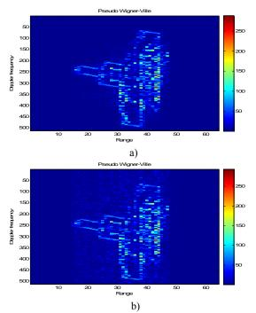
**Fig. 5.** Pseudo Wigner-Ville (PWV) distribution based ISAR image formation for (a) SNR=40 dB and (b) SNR= 10 dB
