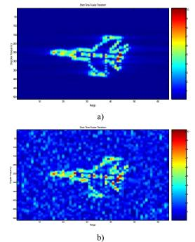
**Fig. 3.** Short time Fourier Transform (STFT) based ISAR image formation for (a) SNR=40 dB and (b) SNR=0 dB
