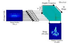
Fig. 1. Time-frequency based image formation
