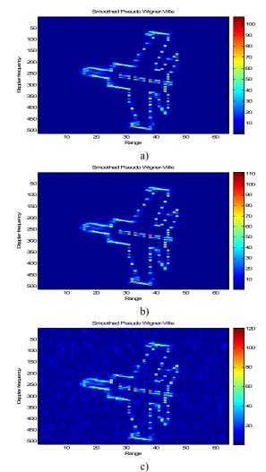
**Fig. 6.** Smoothed Pseudo Wigner-Ville (SPWV) distribution based ISAR image formation for (a) SNR=40 dB, (b) SNR=10 dB and (c) SNR=0 dB
