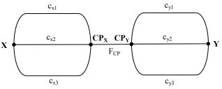
Fig. 6. Representation of the cable system's reliability from EDCR station
