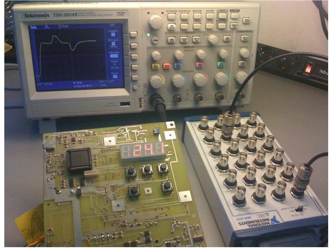
**Fig. 5.** The HIL simulation system for the investigation of aPI controller (the aPI controller is on the left, the connector block of multifunctional PC board PCI-6024E, which is connected to the PC with the installed Simulink software– on the right)
