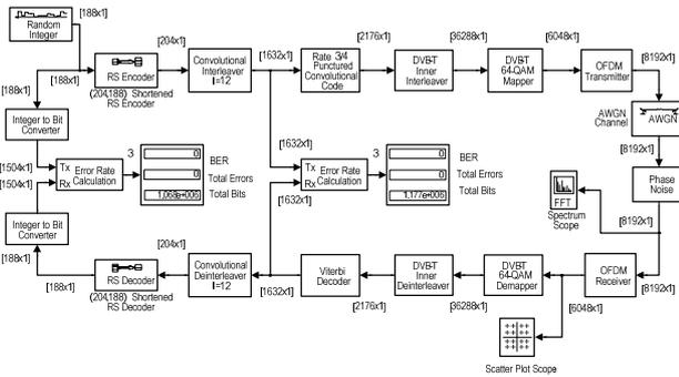
Fig. 3. The model of the DVB-T system
