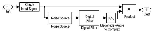
**Fig. 2.** The model of the phase noise generator
