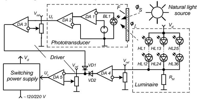
**Fig. 1.** Block diagram of the solid-state lamp. The voltages indicated are the photo-transducer output voltage ( $U_T$ ), power source control voltage ( $U_C$ ), reference voltage ( $V_{ref}$ ), and LED power source output voltage ( $V_d$ )
