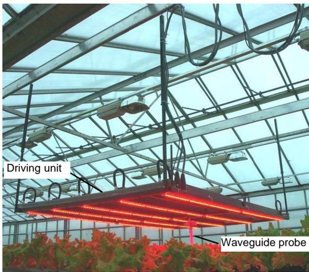
Fig. 4. Solid-state illuminator installed in the greenhouse
