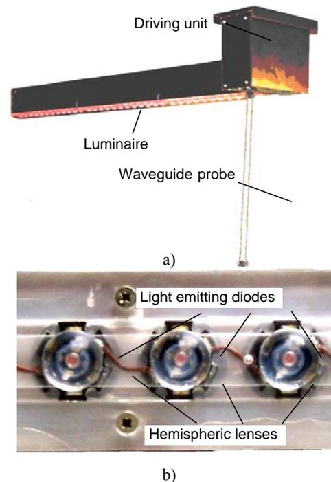
**Fig. 3.** Overall view of the lamp (a); part of the bottom view (b)
