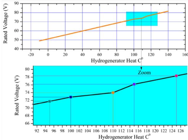
Fig. 1. Exciter voltage variation with hydrogenerator heat
