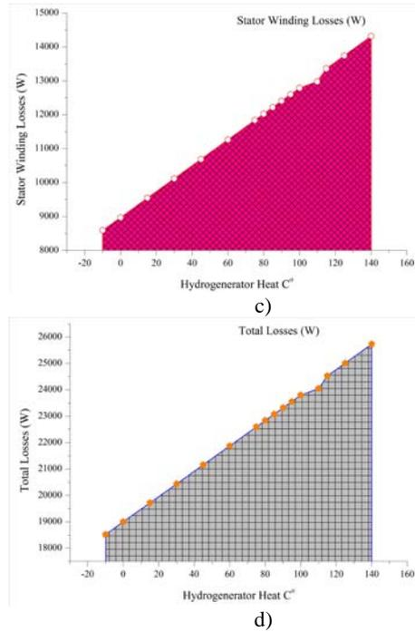
**Fig. 4.** Power losses variation with HG's heat (Watts versus C°): a – field winding losses; b – iron losses; c – stator winding losses; d – total losses
