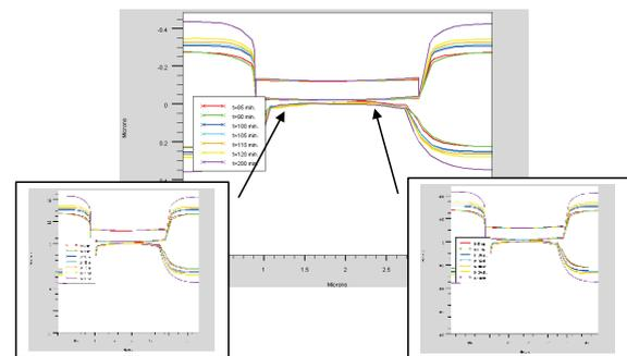
**Fig. 3.** Local oxide profile dependence on the local oxidation process duration (T=1000 °C, SiO<sub>2</sub>=0,02 μm, Si<sub>3</sub>N<sub>4</sub>=0,1 μm, a region length=2 μm)
