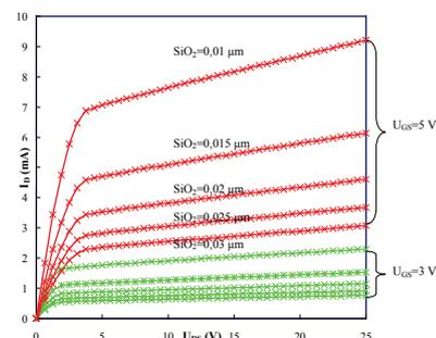
**Fig. 5.** MOS transistor output characteristics ( $L=0,5$   $\mu\text{m}$ ,  $B=3$   $\mu\text{m}$ ,  $U_{\text{GD}}=(3\text{V}, 5\text{V})$ ,  $U_{\text{DS}}=25\text{V}$ ,  $U_{\text{tr}}=1\text{V}$ ) dependence on the silicon oxide thickness, formed before the oxidation process ( $\text{SiO}_2 [0,01\div 0,03]$   $\mu\text{m}$ ,  $t=90$  min,  $T=1000$ °C,  $\text{Si}_3\text{N}_4=0,1$   $\mu\text{m}$ , region length= $2$   $\mu\text{m}$ )
