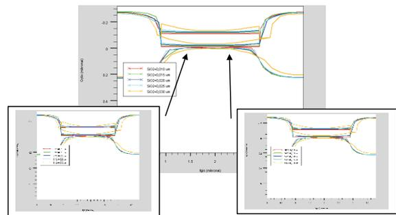
**Fig. 4.** Local oxide profiles dependence on the silicon oxide thickness, formed before the oxidation process ( $t=90$  min,  $T=1000$  °C,  $\text{Si}_3\text{N}_4=0,1$   $\mu\text{m}$ , region length= $2$   $\mu\text{m}$ )
