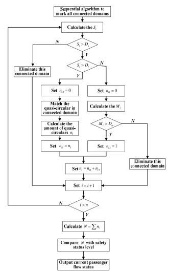
Fig. 5. Procedure of recognition algorithm based on feature of passenger image connected domain.
