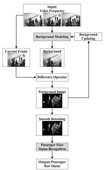
Fig. 2. Basic procedure of passenger flow detection.
