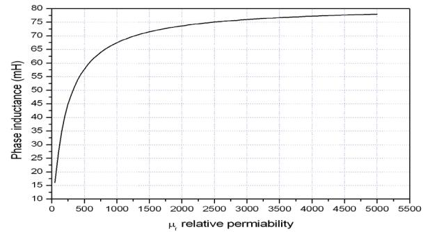
Fig. 8. The impact of relative permeability on inductance
