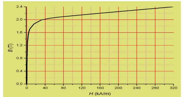
Fig. 3. The  $B$ - $H$  curve of rotor and stator core material
