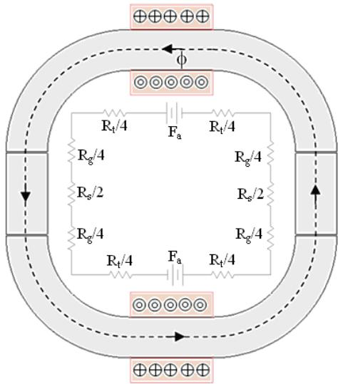
Fig. 5. Actuator core flux path and magnetic circuit
