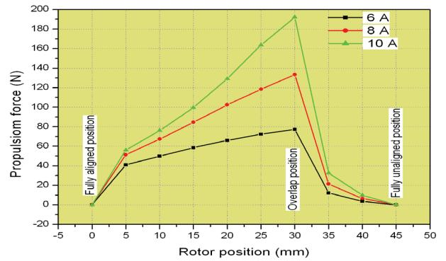
**Fig. 12.** Force profile of the actuator
