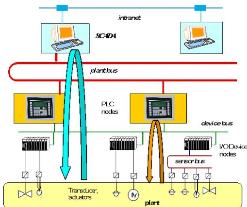
Fig.1. Multilevel structure of the industrial automation system
