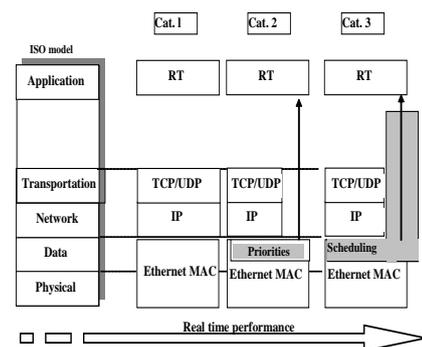
Fig. 2. Classification of industrial Ethernet (IEC 61 784-2)
