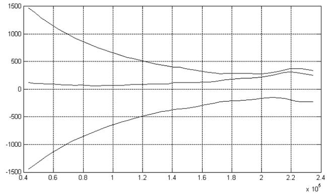
**Fig. 6.** PZT (S3) impedance obtained by the simultaneous multi-frequency method, by using 4x FFT and 1/4 shift of frequency values
