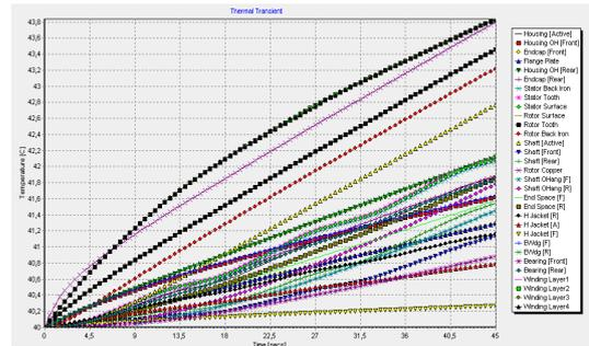
Fig. 7. Thermal values in the different parts of the motor
