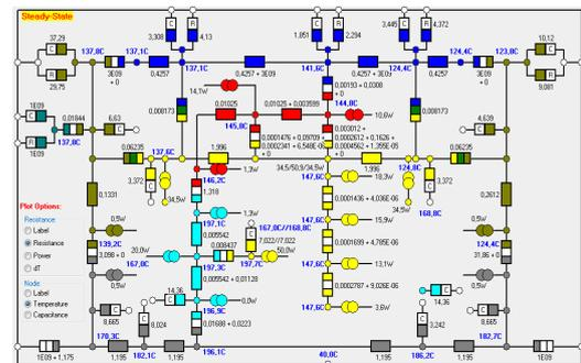
Fig. 8. Steady-state scheme for cast-iron
