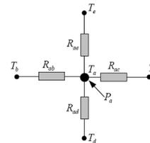
Fig. 1. The basic thermal network constituting the system
