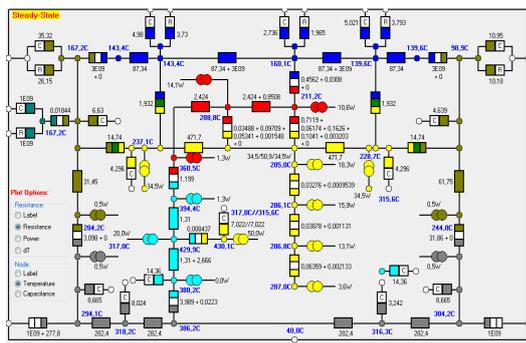
Fig. 9. Steady-state scheme for Teflon material
