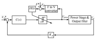
Fig. 5. The fixed frequency self-oscillating control system proposed in [8] and [13].
