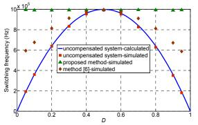
Fig. 15. Switching frequency versus variation of duty cycle: calculated results without frequency compensation, simulated results with proposed frequency compensation, and simulated results with method proposed in [6].
