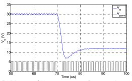
Fig. 13. Partial zoom of the step response of output voltage with the proposed frequency compensator. Top:  $V_o$  (V), bottom:  $V_{pwm}$  (V), the duty cycle is shifting from 0.5 to 0.2 at time 70 µs.
