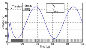
Fig. 14. Output response to a 20-kHz audio reference with the proposed frequency compensator. Top:  $V_o$  (V), bottom:  $V_{pwm}$  (V), the duty cycle is continuously varying from 0.1 to 0.9 and vice versa.
