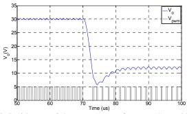
Fig. 10. Partial zoom of the step response of output voltage without a frequency compensator. Top:  $V_o$  (V), bottom:  $V_{pwm}$  (V), the duty cycle is shifting from 0.5 to 0.2 at time 70 µs.
